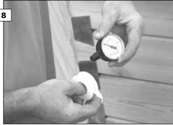
8 Now apply Teflon tape to the outer thread of the manometer.
