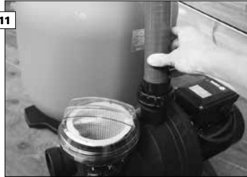
11 Screw the connector pieces into the filter and the pump. Slide the fittings and the inserts over both ends of the hose. Connect the fittings to the connector pieces, and then tighten the fittings. (see the technical section: 2.4.3 Connections)
