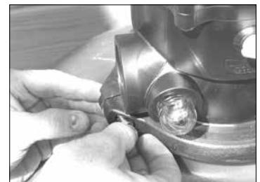
7 The 6-way valve is now placed on the filter and the clamp is fixed around the filter. This is how the valve is connected to the filter.
